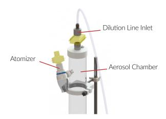
DDS AERO is used to generate aerosolized bacteria for testing Bacterial Filtration Efficiency (BFE).
